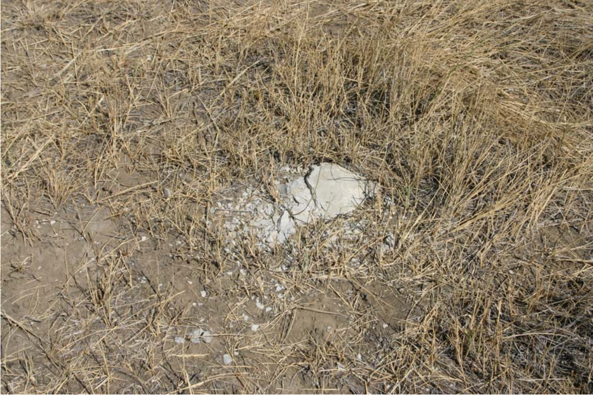
Figure 7. Photo displays the sorts and general surface area of drilling mud and cement found at many well locations within the NWA.
