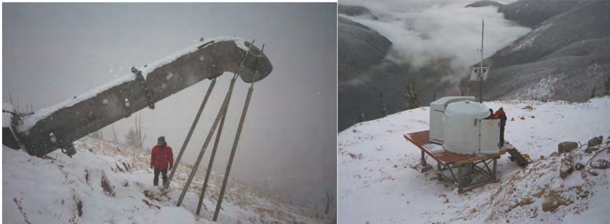
Figure 5.3 Gas-exploder (left) and control shelter (right).
