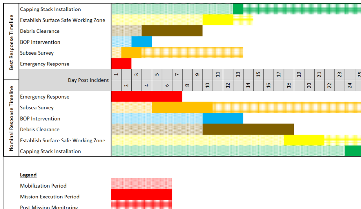
Figure 5: Capping Stack Installation Timeline 13
