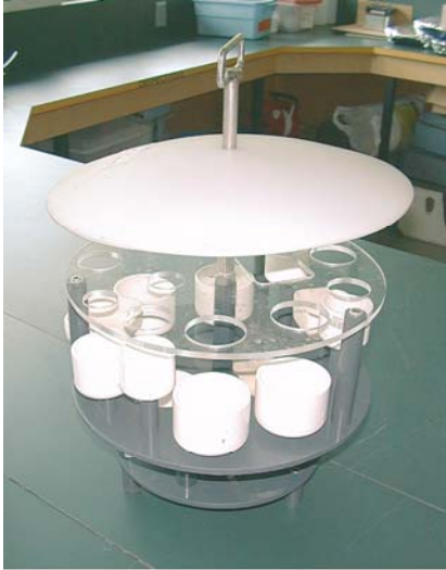
Photo 7. Assembled multi-sampler (Environment Canada and B.C. WLAP (2005 c))
