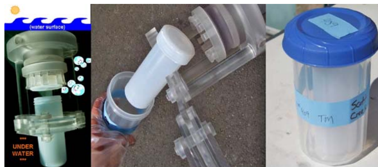
Photo 12. ISOMET sampler under water (Source: Environment Canada (2008 draft))
