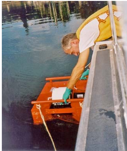
Photo 8. Use of drum roller (Source: B.C. Ministry of Environment (Undated))
