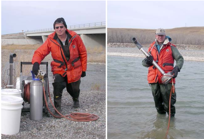
Photo 15. Air lift sampler (Courtesy: Darcy McDonald, Alberta Environment and from Alberta Environment (2006))
