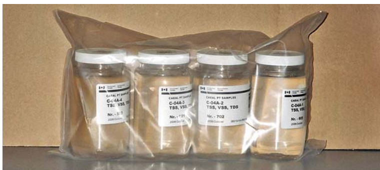
Photo 1. Proficiency testing samples sent to laboratories (Courtesy: L. Swain, Tri-Star Environmental Consulting)
