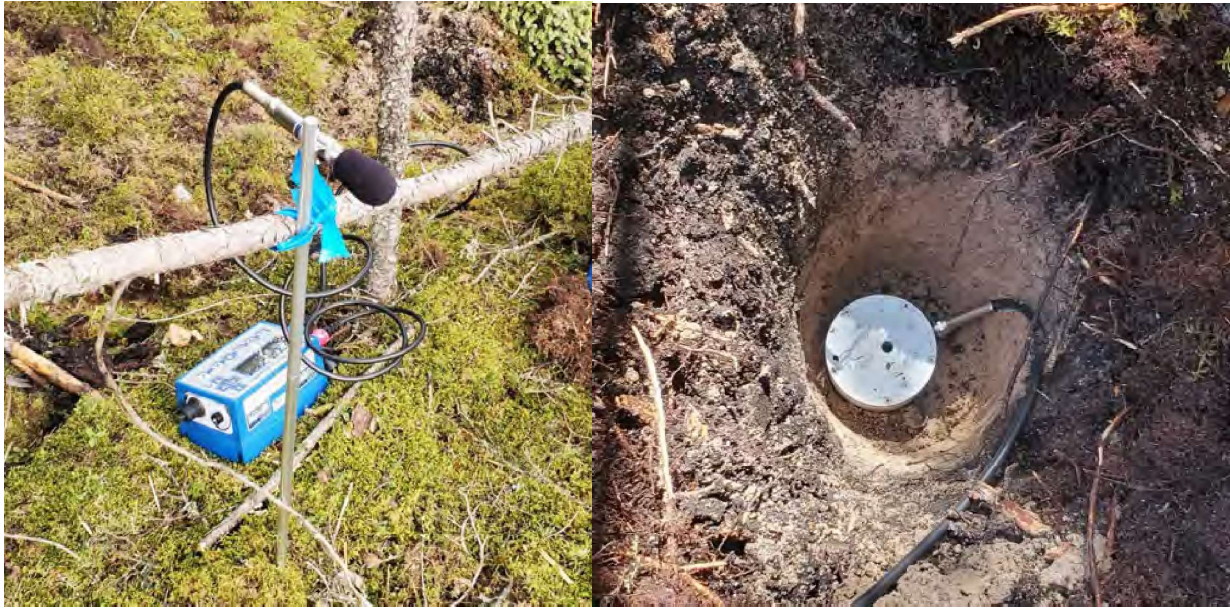
Photo 2.6 Ground Vibration and Air Overpressure Monitoring Setup – May 15
