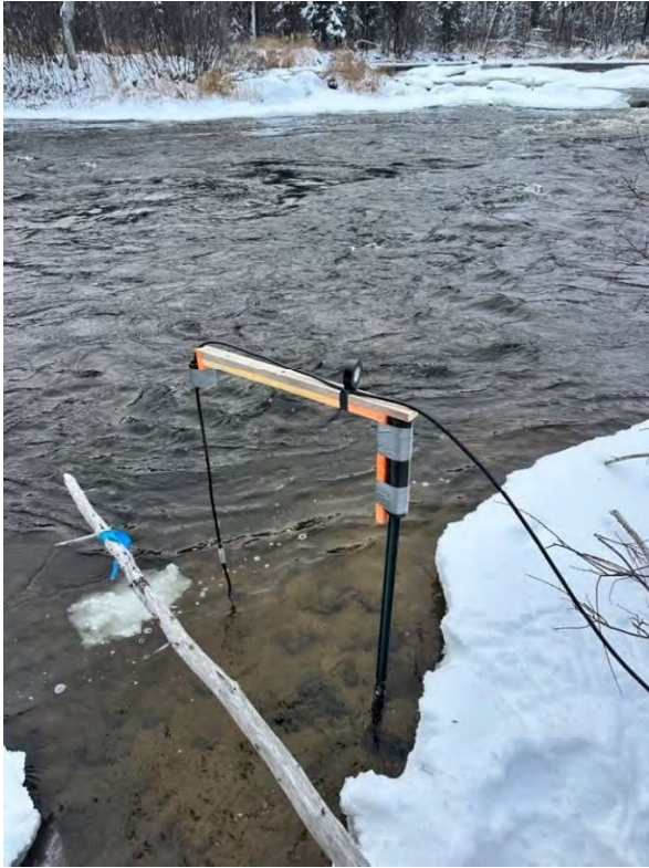
Photo 2.7 Underwater Noise Test Run Setup – November, 2025
