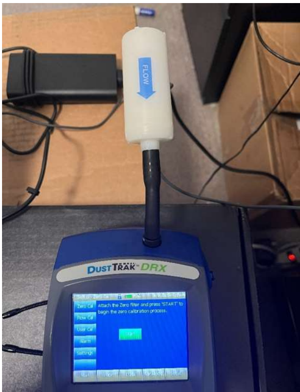
Photo 2.2 TSI DustTrak DRX Model 8534 sampler with zero calibration in progress.
