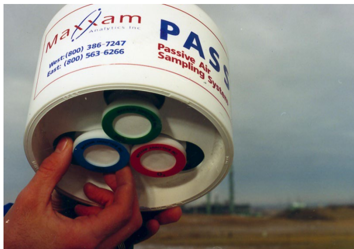
Figure 5 – Installation of Passive Samplers
