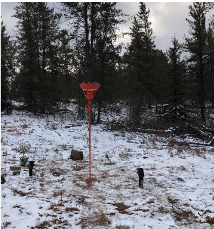
Figure 1 – Dustfall Sampling Stand
